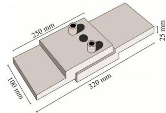
Strain rate = 0.5 mm/min
